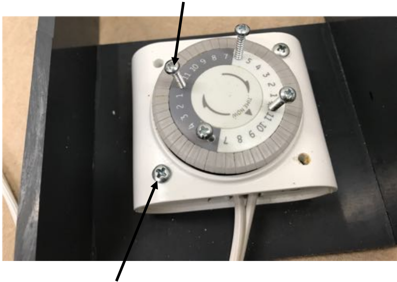
1.5" screws used to fix the timer on the PVC base (two are enough)
